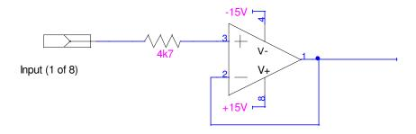
Figure 21. M40 analog input configuration (referenced to AGnd).
