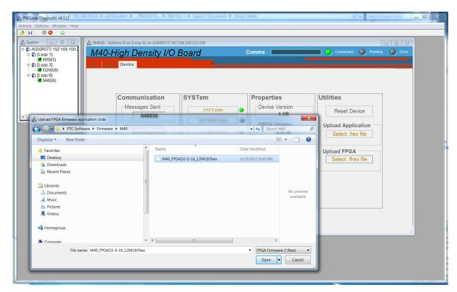
Figure 29. Selecting the flex file to load.
