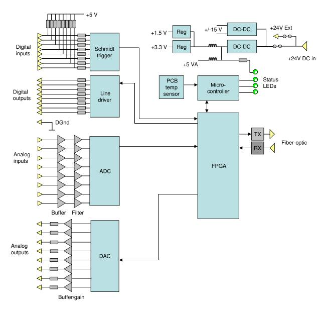
Figure 20. M40 block schematic.
