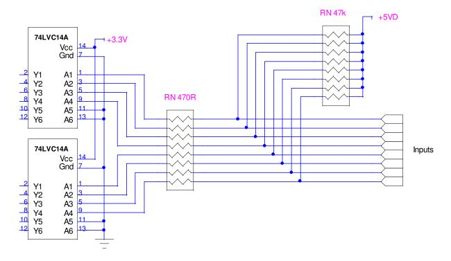
Figure 25. M40 digital input configuration.
