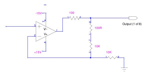
Figure 23. M40 analog output configuration.
