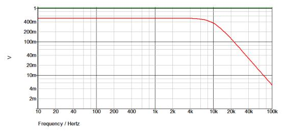
Figure 22. M40 analog input filter response.
