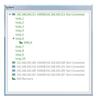
Figure 15. System pane showing M40 connected via A500
