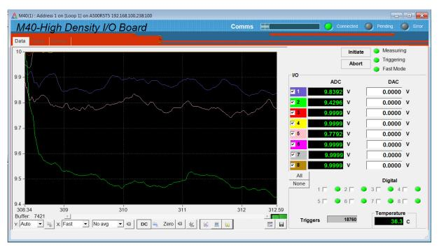
Figure 10. Data tab: M40 running with default settings, showing autoscaled background noise on the inputs.
