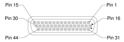
(External view on connector / solder side of mating plug)
