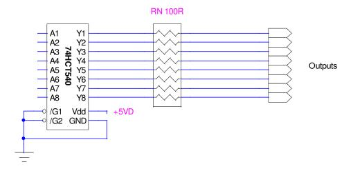
Figure 26. M40 digital output configuration.
