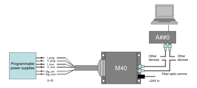
Figure 5. Schematic M40 installation for remote control of a power supply group
