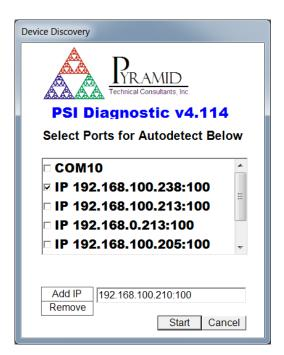
Figure 7. PSI Diagnostic Search Utility – adding a target IP address and port
