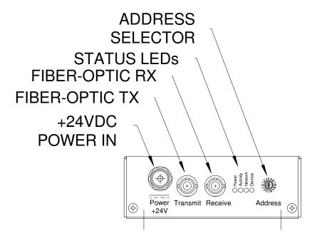
Figure 1. M40 chassis end panels. Dimensions mm.
