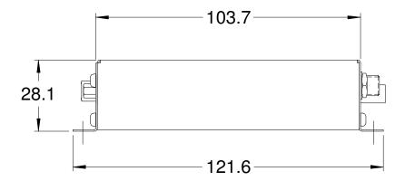
Figure 2. M40 case plan and side views. Dimensions mm.
