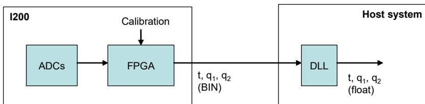
Figure 57. Dataflow in binary mode without A500.
