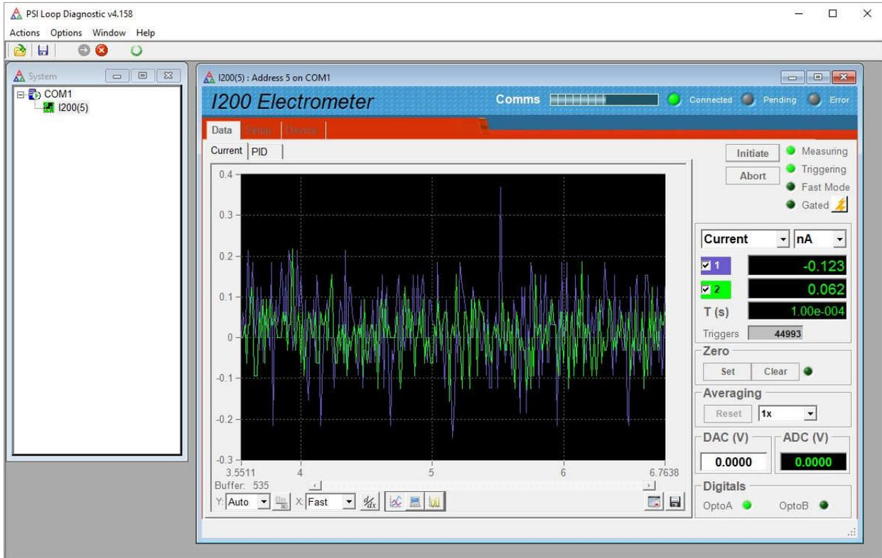
Figure 20. PTC DiagnosticG1 Data tab, strip chart graphic.
