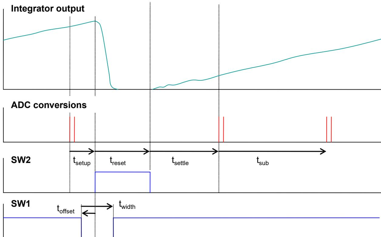
Figure 46. Programmable times for the integrator reset process.
