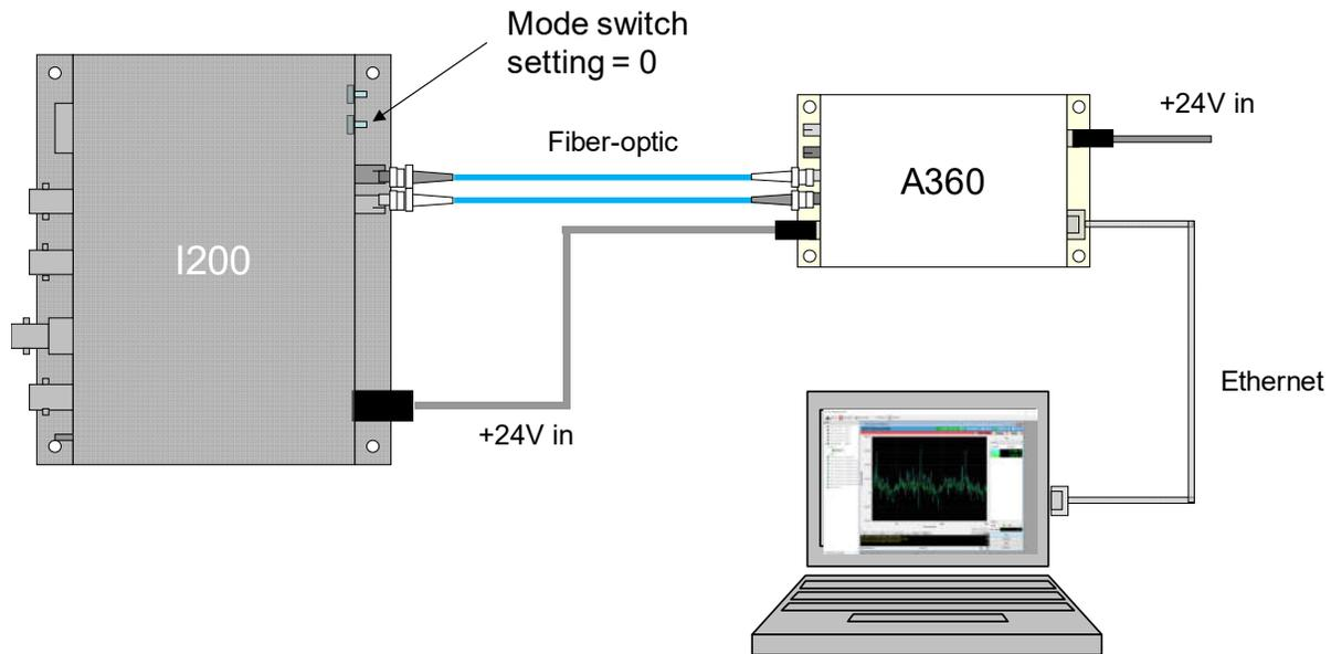
Figure 14. Serial binary connection using fiber optics to A360 and Ethernet to host computer (running PTC DiagnosticG2 host software)
