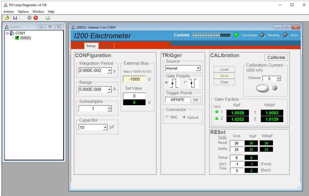
Figure 22. PTC DiagnosticG1 Setup tab showing default settings.
