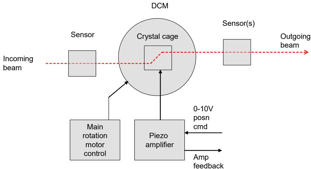
Figure 72. DCM components relevant to servo stabilization
