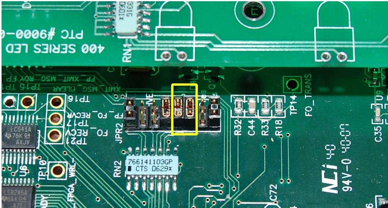
Figure 82. Internal jumper setting for the -100AB option.
