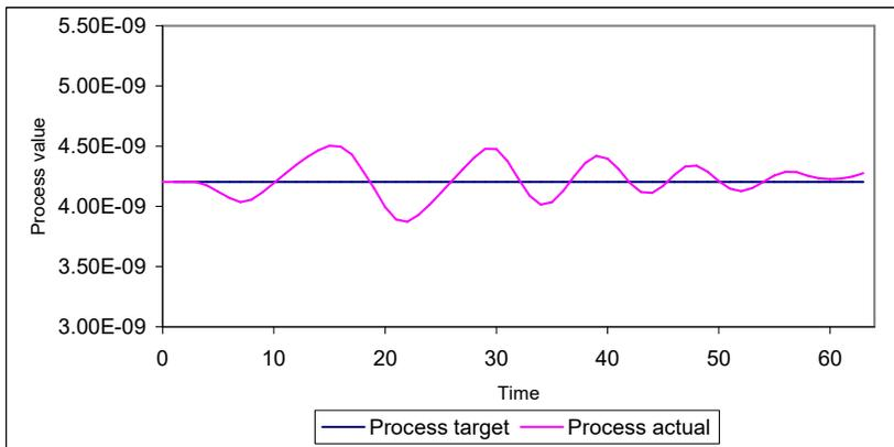
Figure 78. System response with excessive integral servo term.
