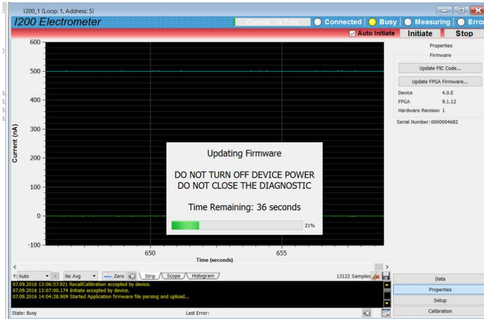
Figure 84. PIC firmware upload in progress (PTC DiagnosticG2).
