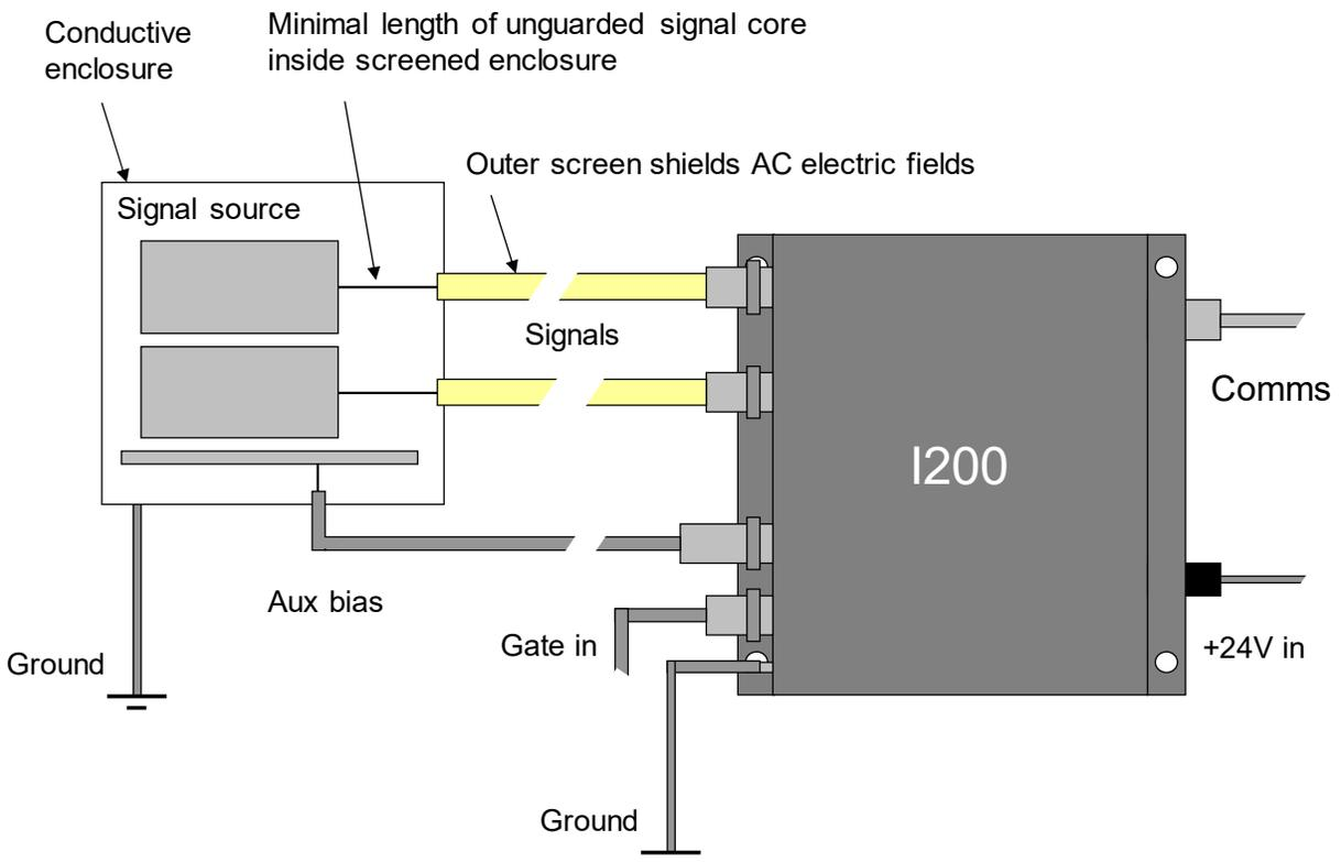
Figure 9. Schematic I200 installation
