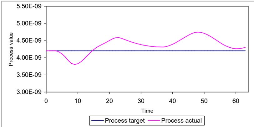
Figure 77. System response with integral servo term.
