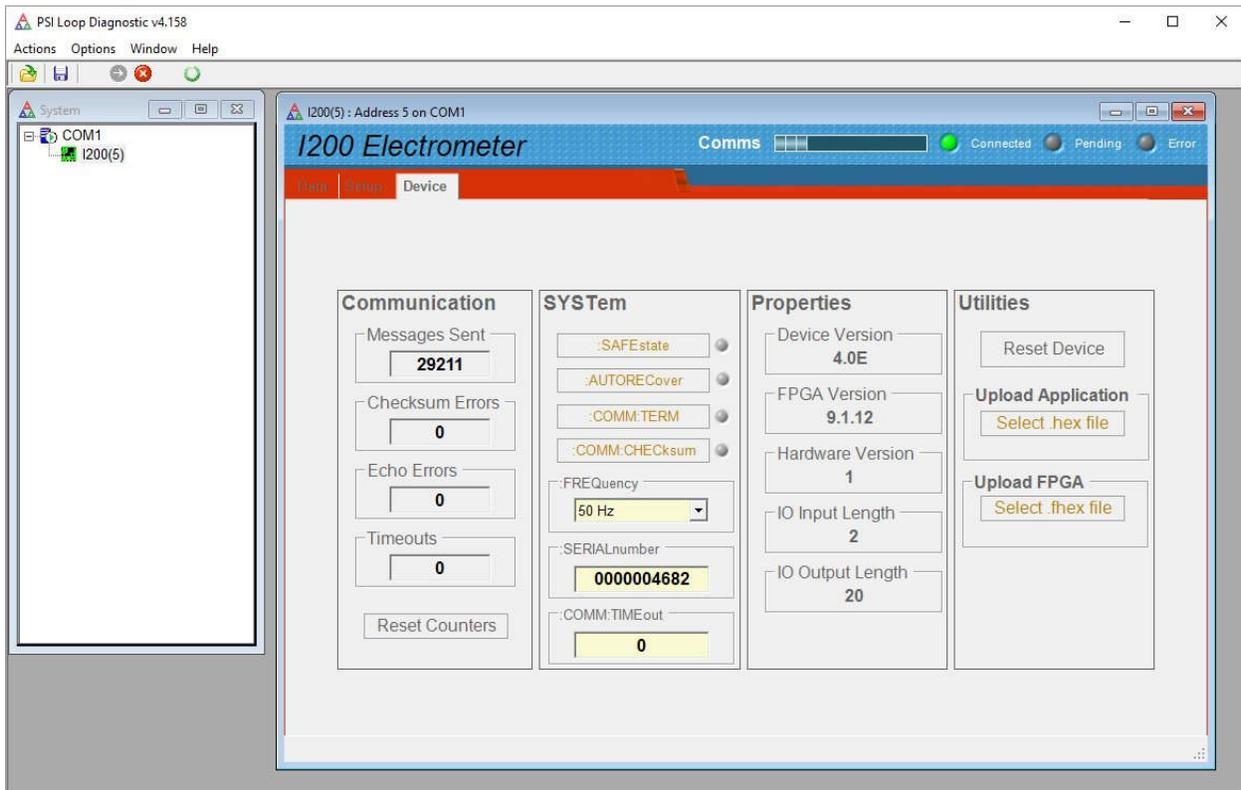
Figure 23. Device tab, showing firmware update utility controls.
