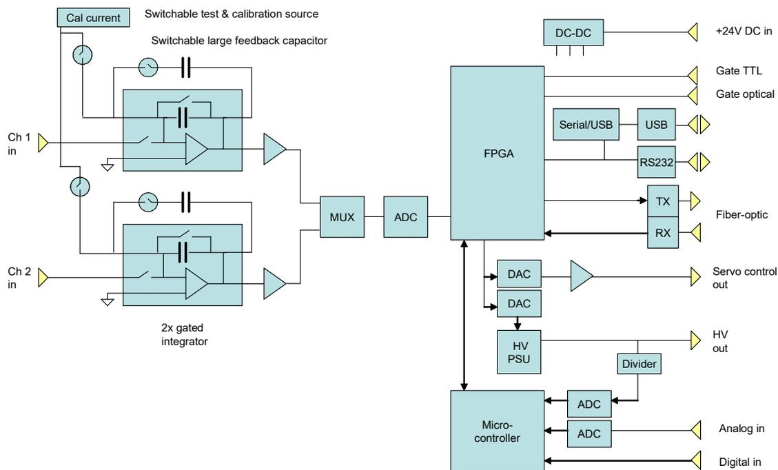
Figure 45. I200 block schematic.
