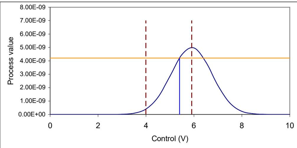
Figure 75. Limits set on control parameter (DAC voltage)
