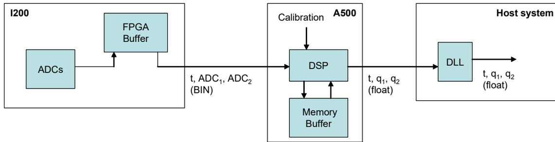
Figure 58. Dataflow in fast binary mode with A500.
