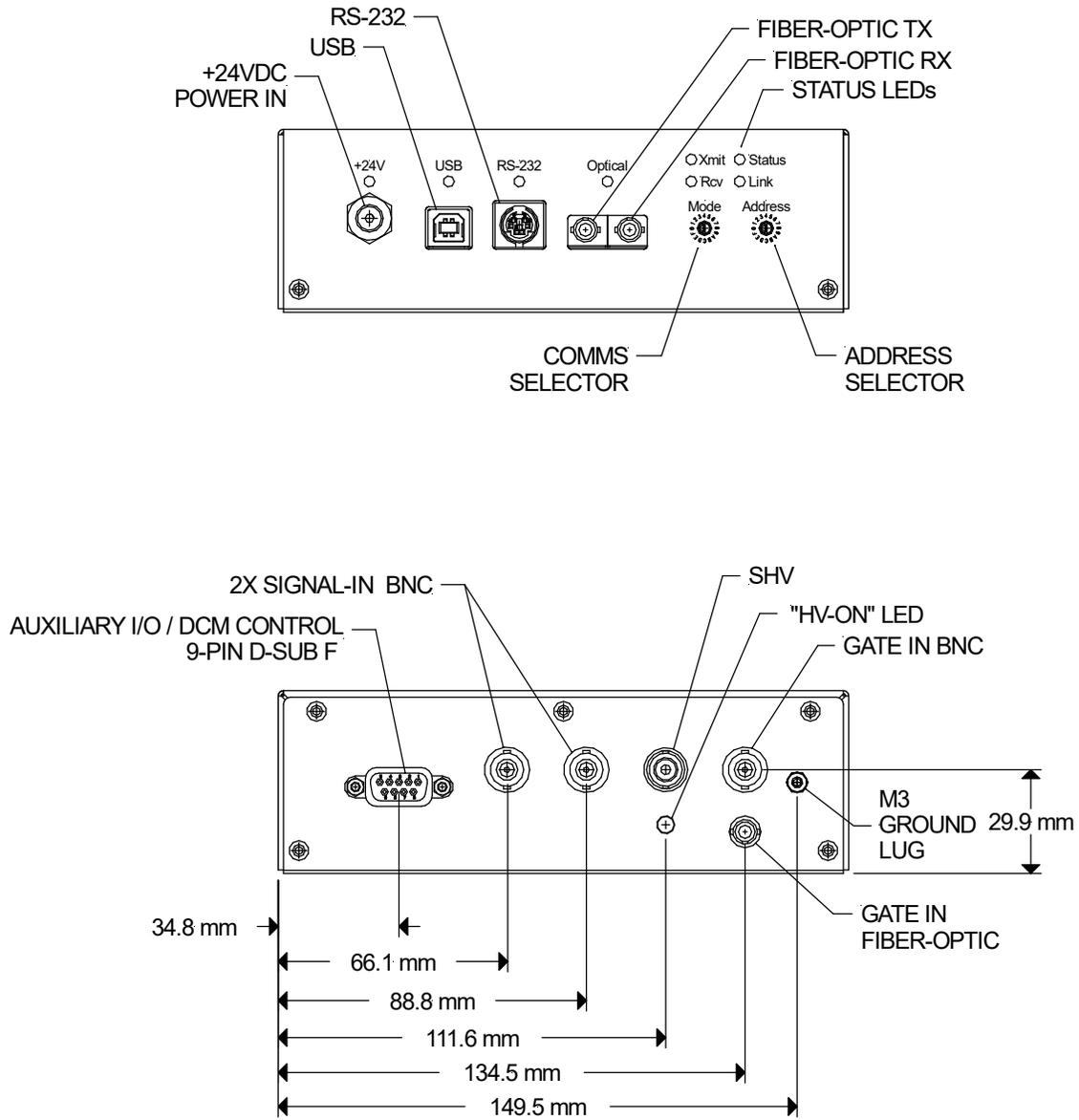
Figure 1. I200 chassis end panels. Dimensions mm.
