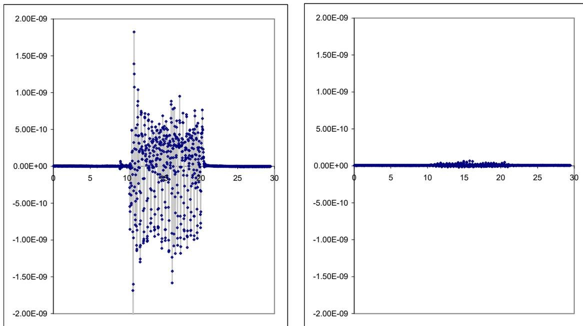
Figure 70. Comparison of triboelectric noise caused by flexing standard RG-58 (left) and low-noise RG-58 (right)
