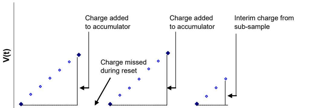
Figure 51. Illustration of integrator voltage at ADC sampling points during charge accumulation. The reset periods are shown relatively large.
