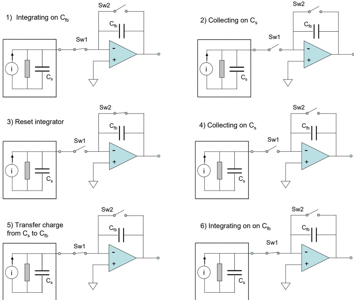
Figure 52. Switching sequence for the no-lost charge method.
