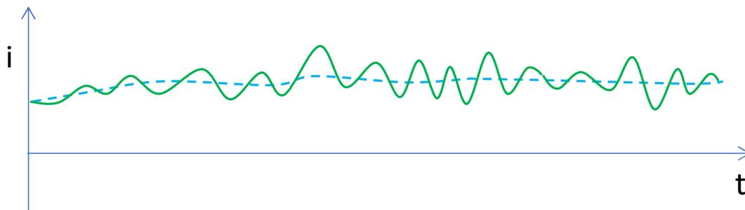
The first example is the most typical. The current varies relatively slowly with time, but there are noise fluctuations superimposed. The value of interest is the moving average (dashed line); we want to filter out the fast noise fluctuations. Both F and U devices are suitable, with F devices preferred if the average signal level is high (100's of  $\mu\text{A}$  or more) and I devices preferred if the signal level is low (below 1 nA).
