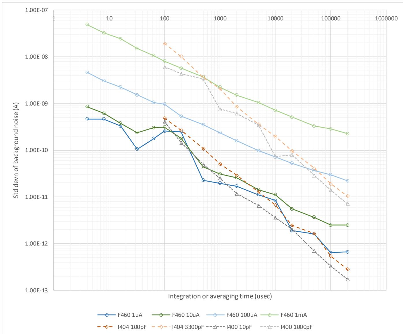
The following plots compare the ability of the F460 and I400 to detect a small current from a miniature ionization chamber connected to one of the inputs. Each device was set to its most sensitive range, and the averaging time or integration time was increased from 1 msec up to 1 second. During the data acquisition a small radioisotope source was placed next to the ionization chamber to provide a measured current of about 40 pA.
