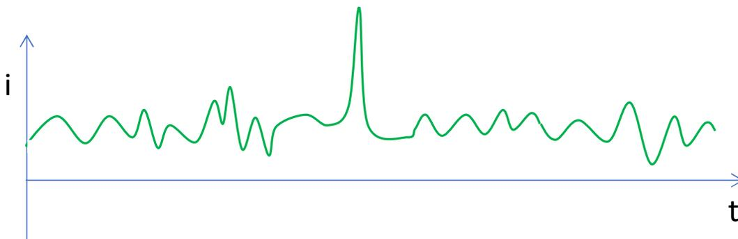
In the second example there is a fast transient event that we wish to record rising above the noise fluctuations. The F device is the appropriate choice. It does not have any reset deadtime which could mask the event, and it is possible to sample the data at a relatively high speed, provided that the current is high enough to avoid the need for much averaging.
