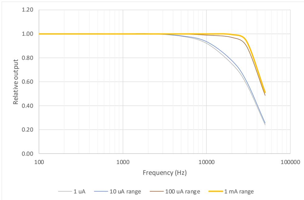
The F device averaging performs block averages of the ADC values, and thus has the same type of frequency response as the I devices. At larger averaging times this dominates, and the same method can be used to suppress line frequency noise.
