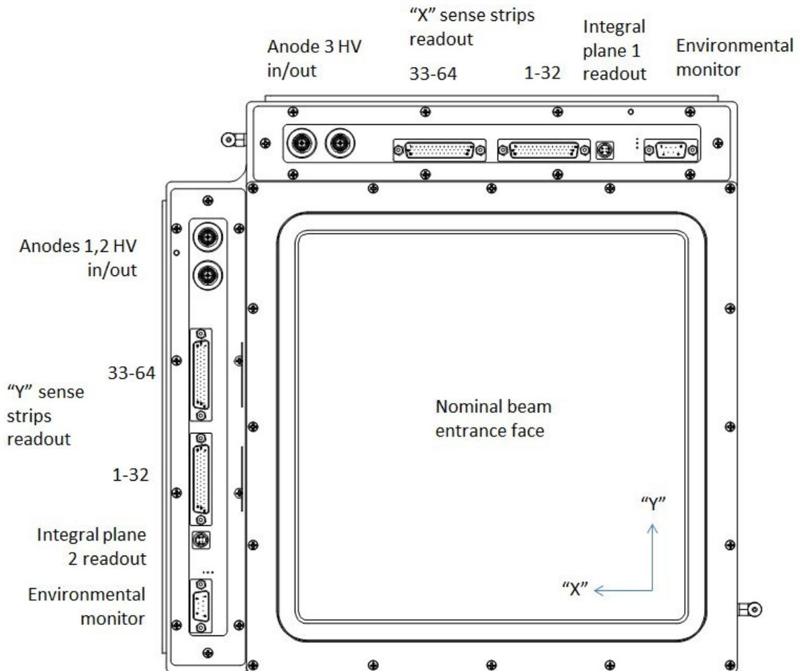
Designation of axes as X / Y, or horizontal / vertical is arbitrary, as it depends upon the orientation of the IC with respect to the beamline. Beam may enter from either direction, entrance face shown is arbitrary, but allows cables to be routed back along beamline.
